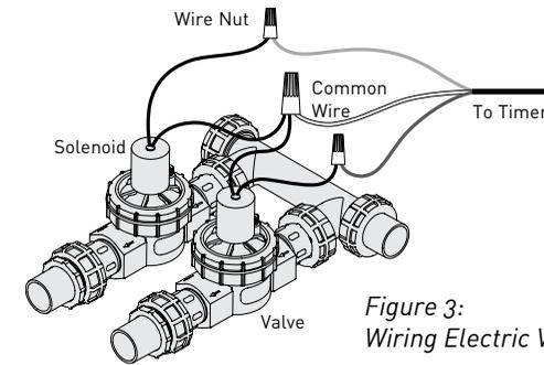
Figure 3: Wiring Electric Valves
