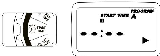
Please note that [START TIME] is the time of day that your programmed watering starts. You can set up to 4 start times at each program if you want to water more than once per day. All stations that have a programmed run time (how long) will run in sequence at each start time.
