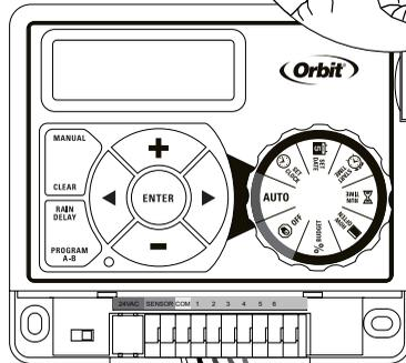
Push tab upward to release wire
